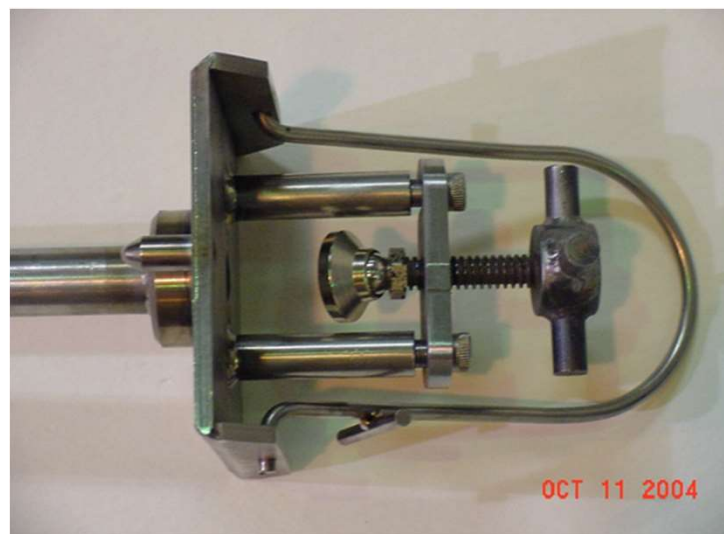
Core sampler swage fixture for new design core sampler.
