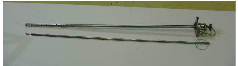
New design core sampler inner and outer tubes with end-cap.
