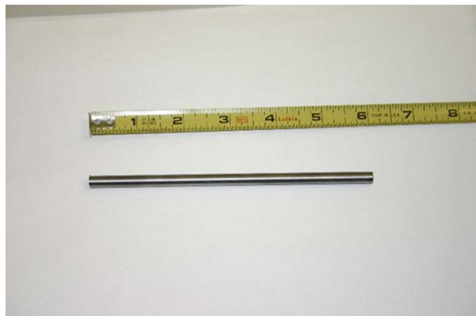
Tantalum filter tube for salt and cadmium sampling.
