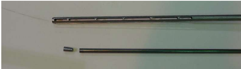
Outer and inner core sampler tubes with interference fit end cap.
