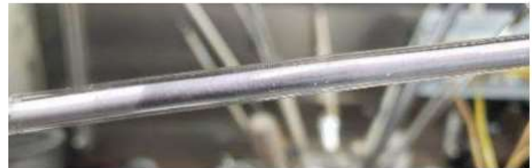
Fines sample taken using a quartz tube. The area to the left is the part touching the bottom of the crucible.
